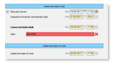
■ In the example, the manual constraint (typically to honour a customer order in time or free a machine) is more restrictive than the constraint imposed by the downstream jobs.
